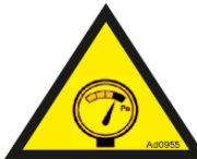
Figure 78 : danger de haute pression.
